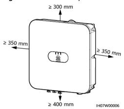
• When installing multiple SUN2000s, install them in horizontal mode if sufficient space is available and install them in triangle mode if no sufficient space is available. Stacked installation is not recommended.
