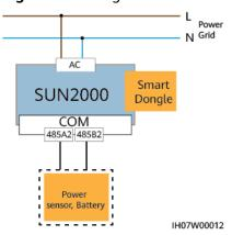
Figure 5-20 Connecting cables to the smart power sensor (single SUN2000)
