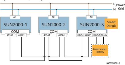
Figure 5-21 In-phase grid connection
