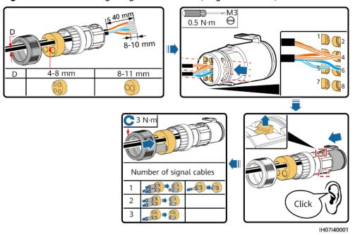
Figure 5-26 Assembling a signal connector (SUN2000 cascading)
