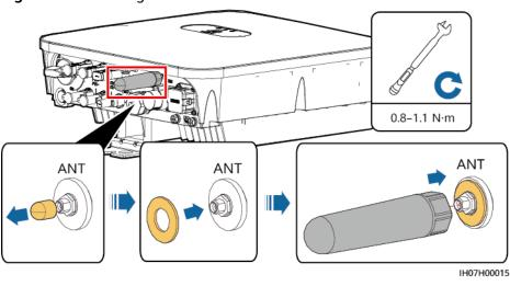
Figure 5-6 Installing a WLAN antenna
