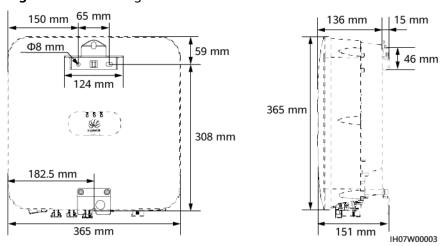
Figure 4-7 Mounting bracket dimensions
