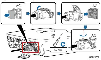
Figure 5-10 Securing an AC connector
