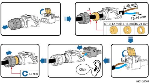
Figure 5-8 Assembling an AC connector (two-core wire)
