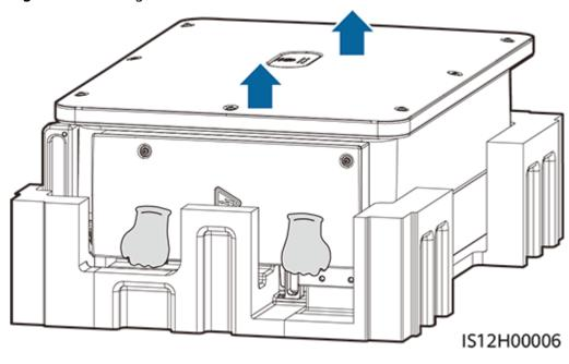
Figure 4-13 Taking out the solar inverter
