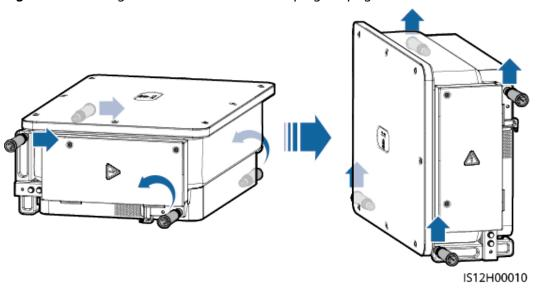
Figure 4-15 Lifting the solar inverter and keeping it upright
