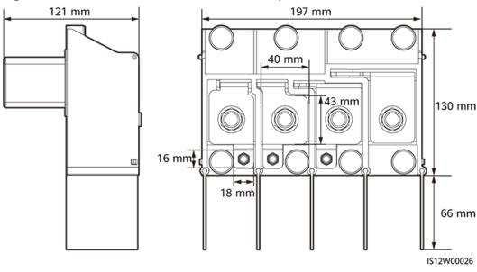
Figure 5-15 AC terminal block dimensions of 4-pin models
