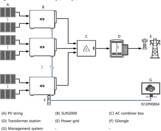
Figure 5-2 RS485 networking (SDongle)
