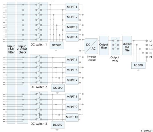
Figure 2-14 Schematic diagram of 4-pin models
