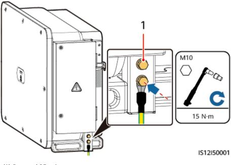
Figure 5-6 Connecting the PE cable to the PE point (on the enclosure)
