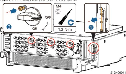
Figure 4-14 Install screws for locking DC switches
