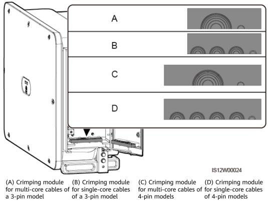
Figure 5-9 Select the crimping module
