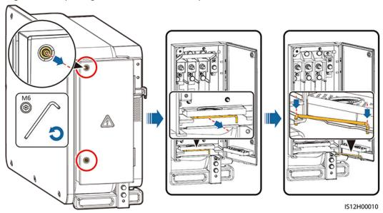
Figure 5-7 Opening the maintenance compartment door
