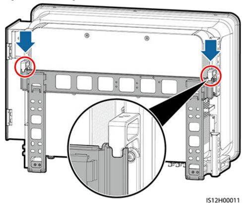
Figure 4-17 Mounting the solar inverter
