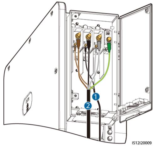
Figure 5-12 Cable connection sequence
