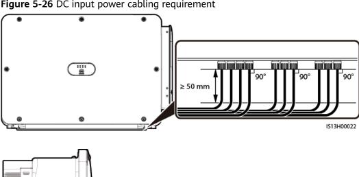
Figure 5-26 DC input power cabling requirement
