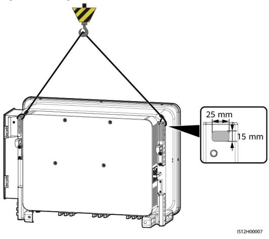
Figure 4-16 Hoisting the solar inverter
