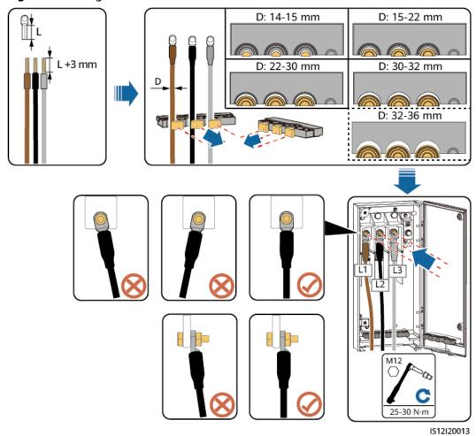
Figure 5-17 Single-core cable connections
