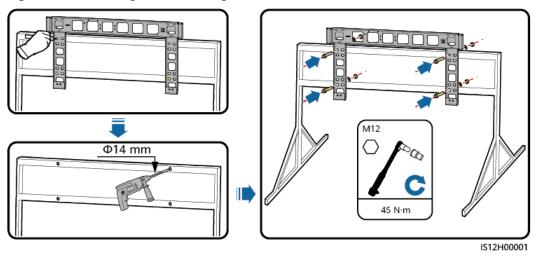
Figure 4-9 Installing the mounting bracket
