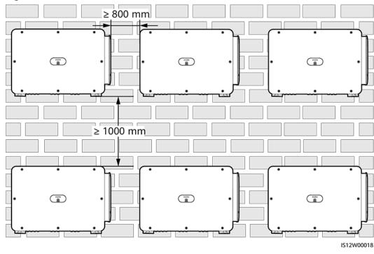
Figure 4-6 Stacked installation mode (not recommended)
