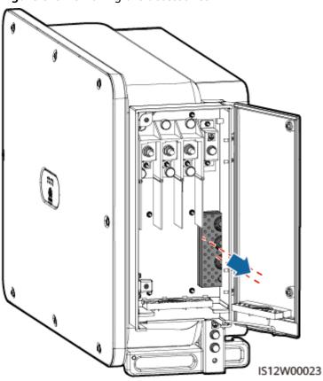
**Figure 5-8** Removing the accessories
