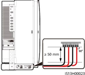
During DC input power cabling, leave at least 50 mm of slack. The axial tension on PV connectors must not exceed 80 N. Radial stress or torque must not be generated on PV connectors.
