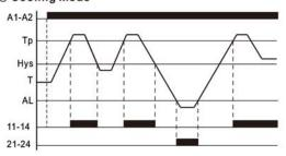
After energization, if measured temperature T is higher than the set temperature Tp, output contact 11 and 14 switch ON; when the measured temperature T drops to the "Hys" position, output contact 11 and 14 switch OFF.
