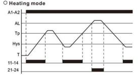
After energization, if measured temperature T is higher than the set temperature Tp, output contact 11 and 14 switch OFF; when the measured temperature T drops to the "Hys" position, output contact 11 and 14 switch ON.
