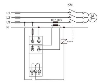
Note: It is possible to increase the current range of RS-MI by using an external current transformer if measured current exceed 10A
