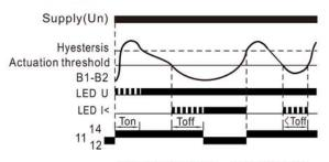
Ton: Start-up delay Toff: Trip delay
